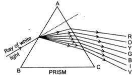
(b) In the glass slab has opposite sides are parallel but in prism the opposite sides are at some angle.
