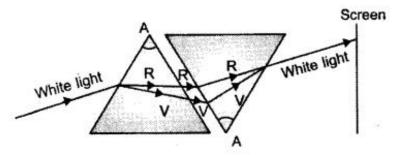
4 What is dispersion of white light? What is the cause of such dispersion? Draw a diagram to show the dispersion of white light by a glass prism. (b) A glass prism is able to produce a spectrum when white light passes through it but a glass slab does not produce any spectrum. Explain why is it so?
